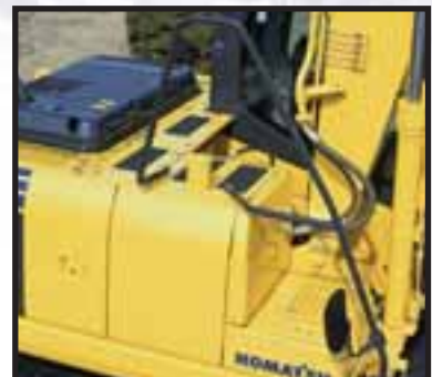
Large handrail for safe access
