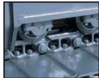
Track link with strut The PC130-7 uses track links with struts, providing superb durability
